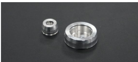
Payne Diffusion Cell: Small (9mm) and Large (18mm, only for high mass balance configuration).
