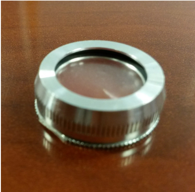
Figure 7 – Payne Cell filled with sample.
