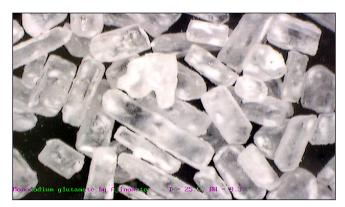
Figure 3. Video microscopy output on monosodium glutamate at 0%RH and 25  $^{\circ}$ C.
