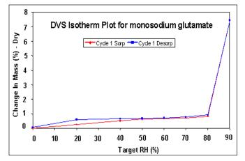
Figure 2. Water sorption isotherms for monosodium glutamate at  $25^{\circ}$ C
