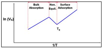
Figure 2. Schematic Diagram of iGC SEA retention around the  $T_a$  (from [1]).
