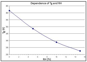
Figure 4. Experimentally obtained glass transition temperatures in dependence of relative humidity (with decane).
